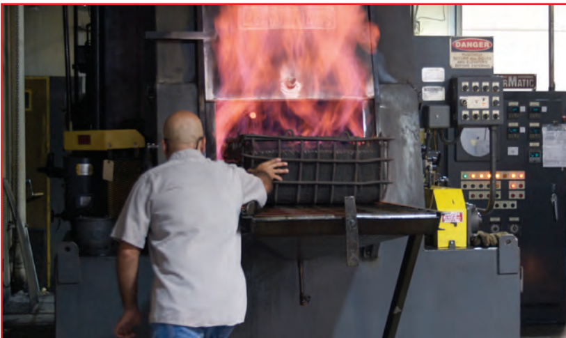
Heat-treating is critically important in obtaining the correct tensile strength. Fasteners are placed in special vertical racks to ensure complete 360° penetration.
