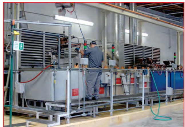
The finishing touch for most chrome moly fasteners is the black oxidizing operation. Fasteners go through a series of "baths."
