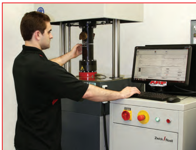
ARP has two highly sophisticated Ansler fatigue machines, which test fasteners through millions of cycles.
